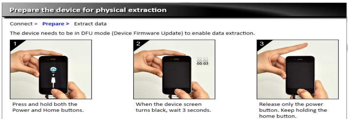
Screenshot 5.1 Preparing iPhone phone for physical data extraction
