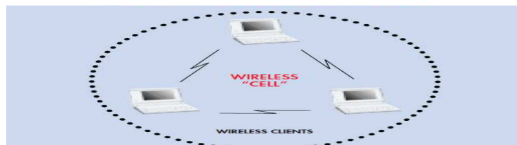
FIGURE 2.2: Peer to peer configuration (DDS, 1999)
